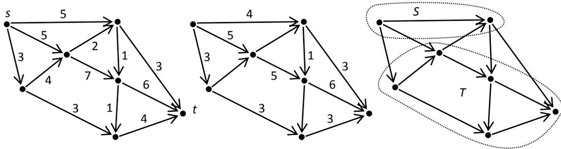
Figure 1: Left: A directed graph with edge capacities. Center: A maximum flow. Right: A minimum cut.
